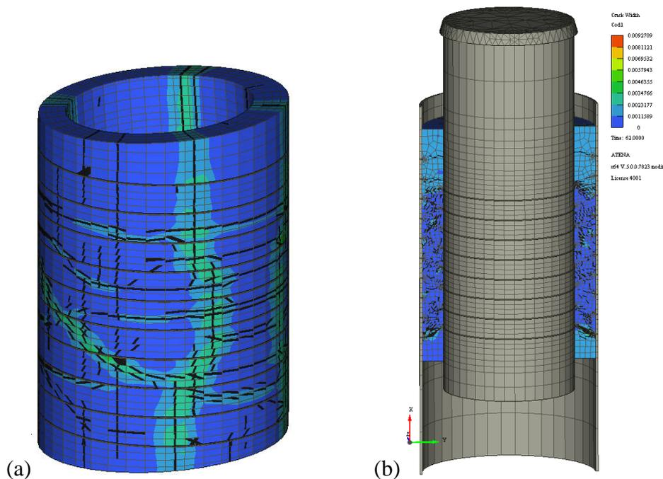
**Fig. 5** (a) Shrinkage cracks (b) the final failure mode at peak load
