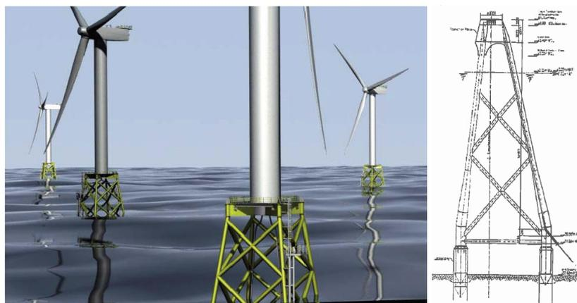
Fig. 1 The typical geometry of the support structure of offshore wind power plants
