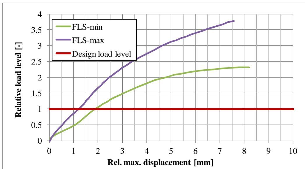
**Fig. 6** Load-displacement curve for the global fatigue assessment
