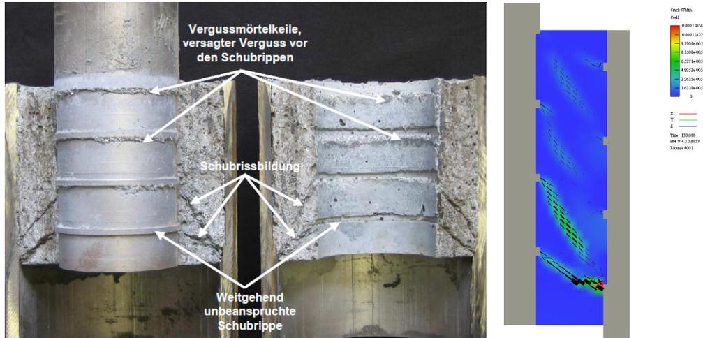
Fig. 6 Failure mode in (a) experiment (Anders [3]) (b) analysis by ATENA
