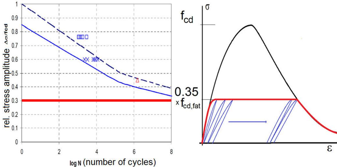
**Fig. 2** Limit stress value according to [4] and its application as a modified stress-strain law
