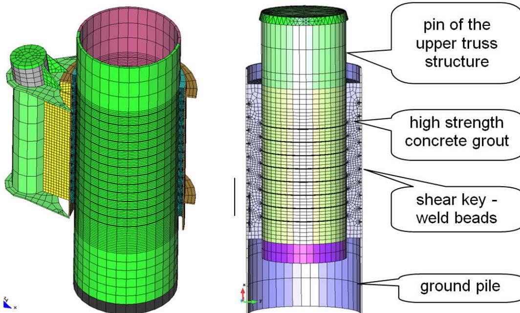
**Fig. 3** The finite element model for two types of grouted connection
